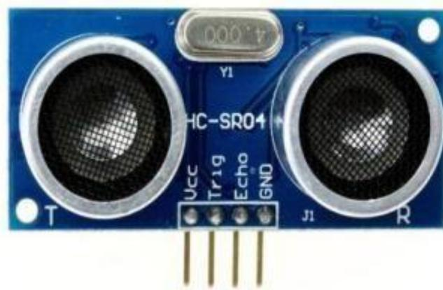
Gambar 4. Sensor Ultrasonik
