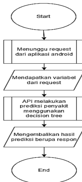
Gambar 3. Flowchart API (Application Programming Interface)
