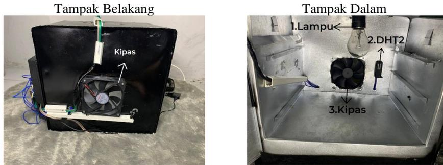
Gambar 4. *Prototype Smart Oven*
