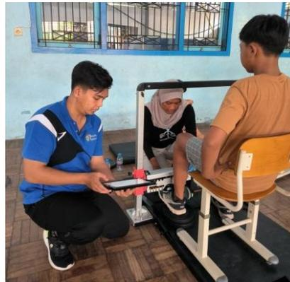
**Gambar 3. Ankle Plantar Flexion Test**
