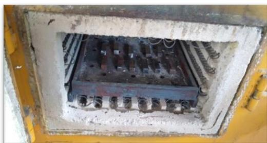
Gambar 4. Baja dilakukan proses *heat treatment*.
