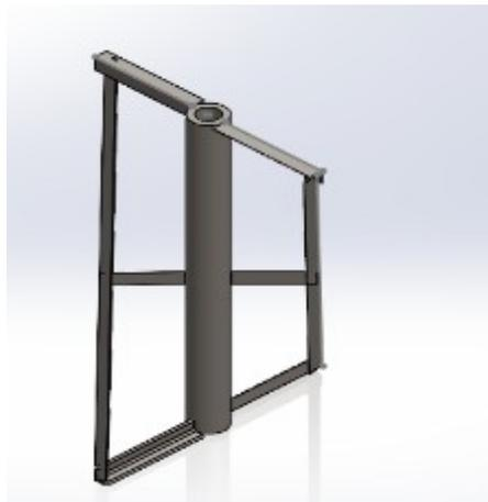
Gambar 2 Blade mixer tampak isometri
