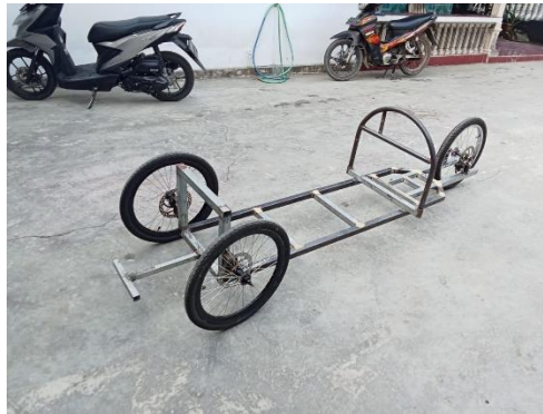
Gambar 3. chassis mobil listrik
