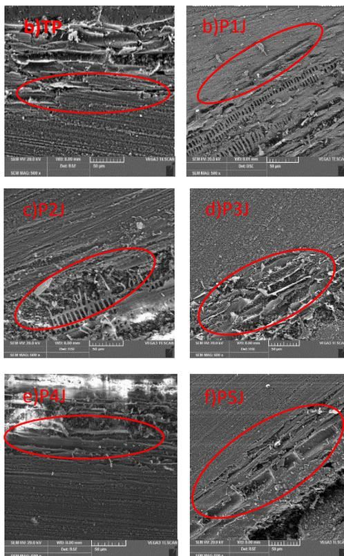
Figure 2. Observation of compatibility between fiber and matrix : a) not treated b–f) treated
