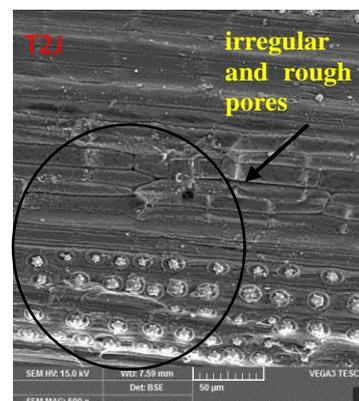
Fig. 1c. Fiber surface with 2 hours immersion treatment
