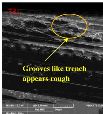
Fig. 1d. Fiber surface with 3 hours immersion treatment
