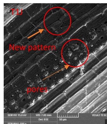
Fig. 1b. Fiber surface with 1 hours immersion
