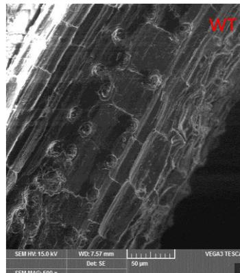
Figure 1a. The fiber surface of the untreated fiber
