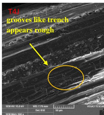
Fig. 1e. Fiber surface with 4 hours immersion treatment
