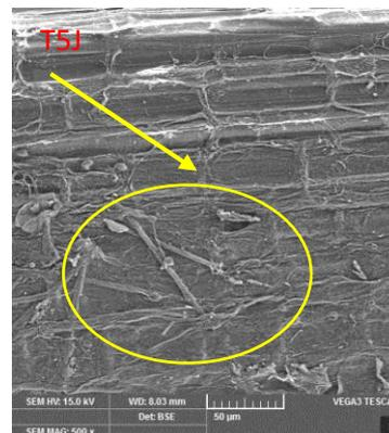
Fig. 1f. Fiber surface with 5 hours immersion treatment
