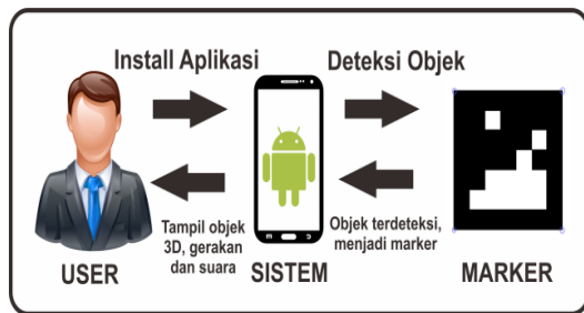
Gambar 1. Cara Kerja Sistem Augmented Reality
