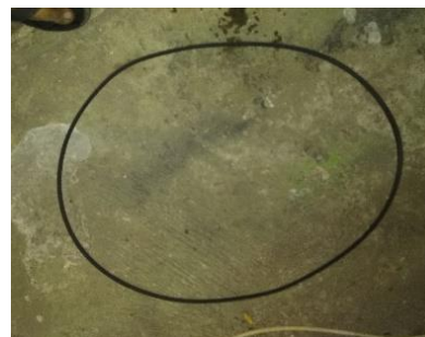
Gambar 5. V-belt 79 inci tipe A
