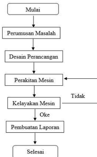
Gambar 4. Diagram Alur Prosedur Perancangan.
