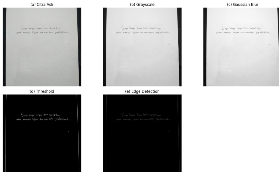
Gambar 6. Hasil preprocessing citra: (a) citra asli, (b) grayscale, (c) Gaussian blur, (d) thresholding, dan (e) edge detection.
