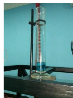
Gambar 6. Flowmeter bahan bakar
