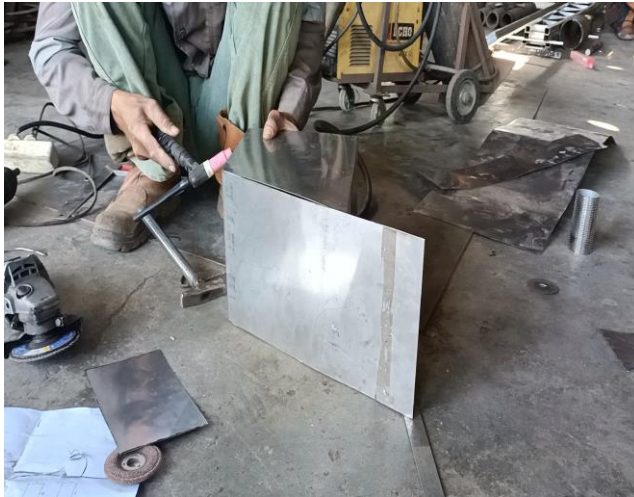
Gambar 7. Proses pengelasan cover parut
